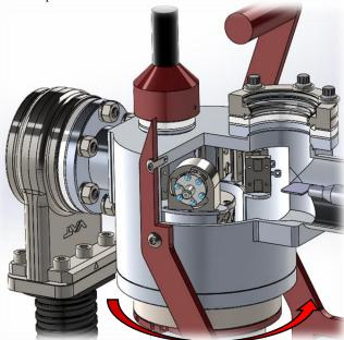
Cutaway view showing the arrangement of 6 sample docks.
